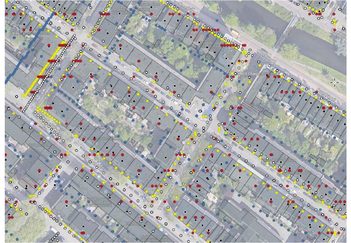
(left) 5 different geocode providers. All describe the same objects, none of the geocodes are the same.
